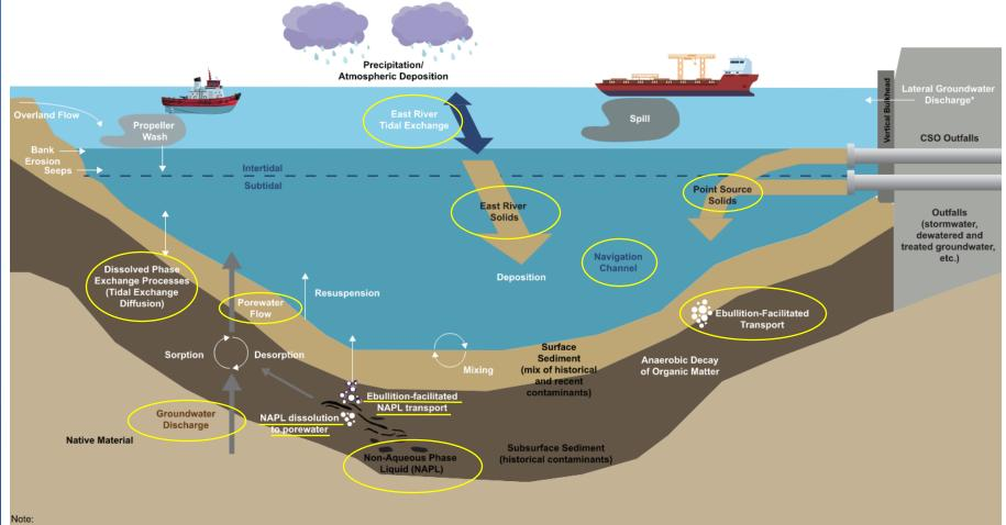
This figure is intended to illustrate ongoing external inputs of solids and contaminants to the East Branch and in-creek processes that affect the redistribution of solids and contaminants in the East Branch. \*Lateral groundwater discharges occur in vertical permeable shoreline areas that include vertical wood, wood, precast concrete, and pile-supported concrete bulkheads.
